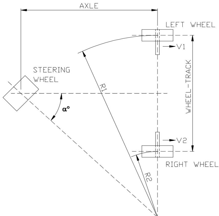
The relationship between the two motors speed is equal to the relationship between the two radius described during the curve.
