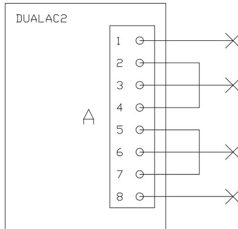
Bridge 2-4 and 5-7 connect both built-in 120 ohm can termination resistances.
