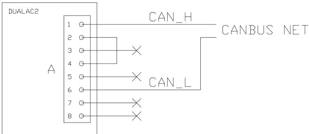
Bridge 2-4 connects one built-in 120 ohm can termination resistance, the second will be connected in another module of the canbus net.
