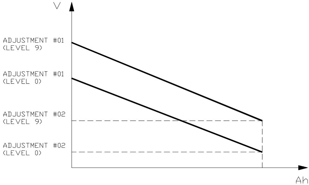
15 MAIN CONT VOLTAGE: this parameters adjusts the Line contactor coil voltage (PWM output C26)
