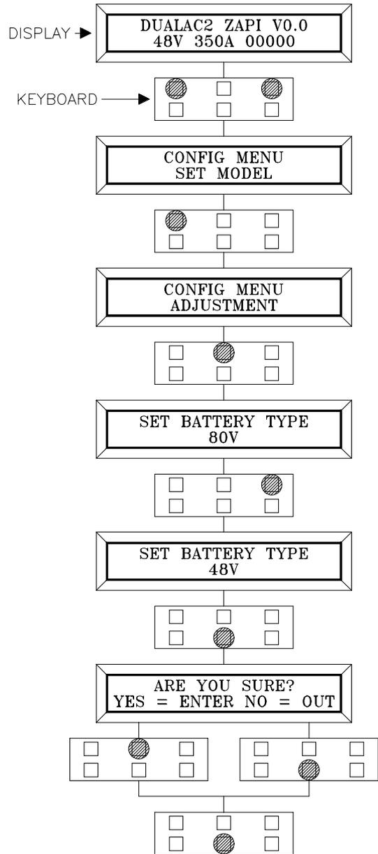
Flow chart showing how to carry out ADJUSTMENT BATTERY operation by console.
