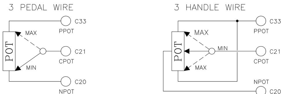
PPOT is the accelerator unit positive supply. It can be either a 5V output or a 10V output. The selection of the output voltage is made in the logic card by moving a jumper (factory set).
