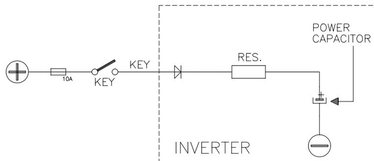
When the key is switched ON, the inverter tries to charge the capacitor through a power resistance, and check if the capacitor are charged within a timeout. If they do not charge, an alarm is signalled; the main contactor is not closed.
