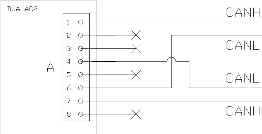
The canbus built-in termination resistances are not inserted.
